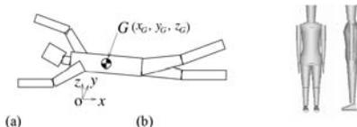
Figure 1. Modeling of a swimmer's body. (a) Analytical model of a self-propelled swimmer. (b) Example of the modeled body for averaged Japanese 20-29 years old male.
