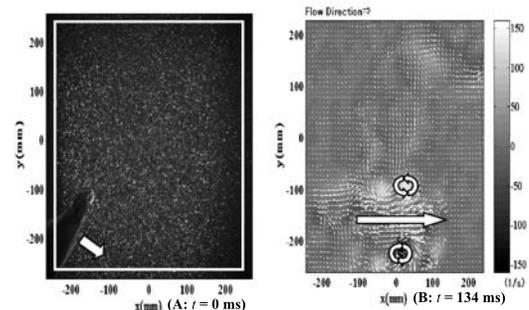
Figure 2. An exemplary image of downward dolphin kicking motion (tiptoe image, A:  $t = 0$ ) and the velocity-vorticity map (B:  $t = 134$  ms). The white rectangle in the left panel corresponds to the right panel. The grey scale indicated in the right column denotes the magnitude of vortices.
